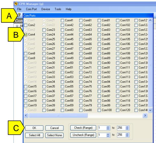
Now click on Com4 (Arrow D) and a set up window should appear to the right. The presets are in place and require no alteration on your part, but you will have to enter an address of the controller down in the service host box. If you want to test your installation, use the unit at the Lakewood Instruments factory. Its IP address is 75.19.65.62 and its port is 10001. Enter it as shown below (Arrow E) and then click the save icon again (Arrow F).
